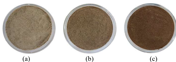
Fig. 1: Corn silk powder obtained by (a) lyophilization (b) tray drying at 60°C and (c) tray drying at 40°C.
