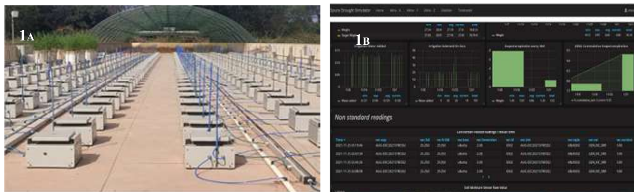
Fig. 1: (A) High throughput phenomics facility established at Department of Crop Physiology, University of Agricultural Sciences, Bangalore. (B) Automated software controlled system enables the measurement of hourly transpiration and cumulative water transpired.
